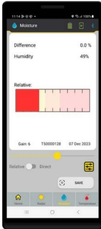
Figure 22 Relative Moisture Sensor
