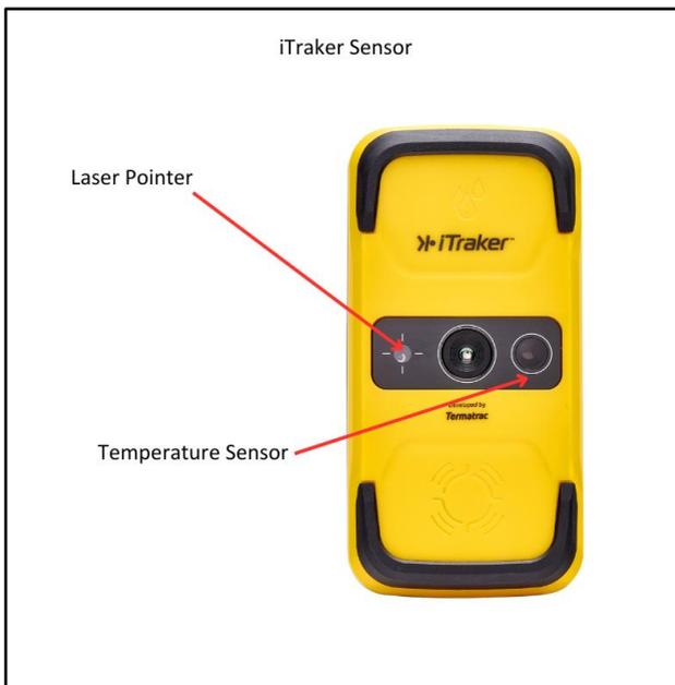
Figure 12 iTraker and Temperature Sensor
