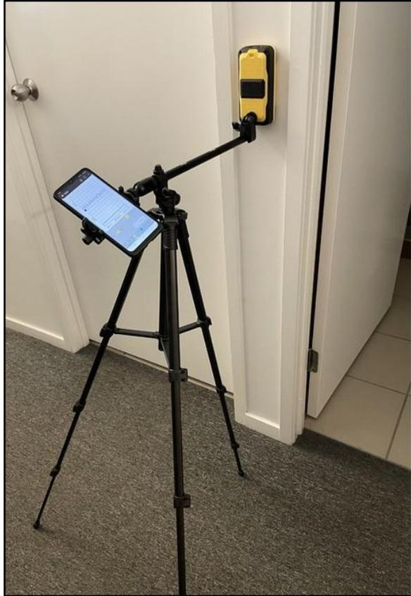
Figure 6 Tripod against Wall - Radar Sensor
