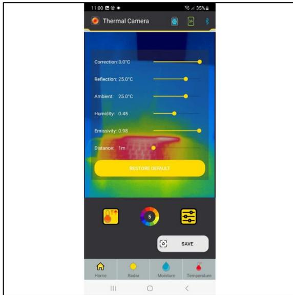
Figure 39. Thermal Camera Settings on the iTraker App
