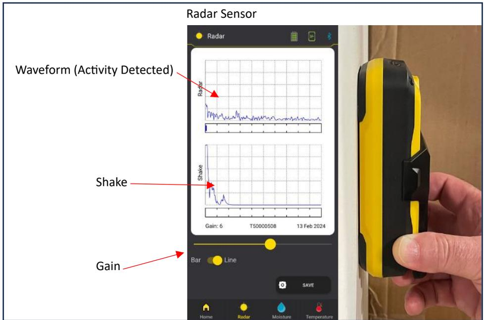
Figure 9 iTraker and Radar Data
