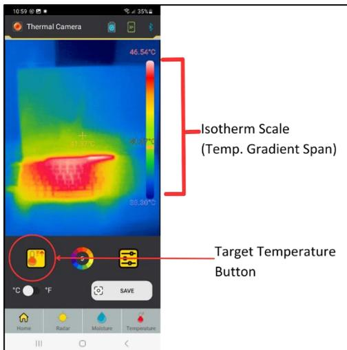
Figure 42. Surface Temperature Reading
