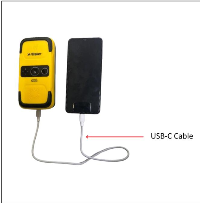
Figure 36. USB-C Type Cable to connect the iTraker PRO and Mobile Phone
