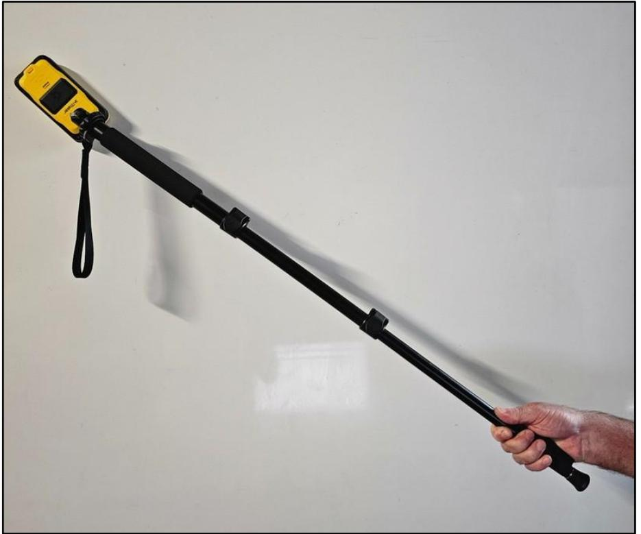
Figure 7 Monopod held to the wall- Direct Moisture Sensor
