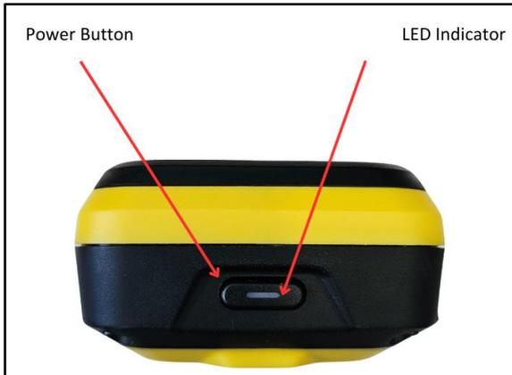
Figure 15 iTraker Button and LED Indicator Locations
